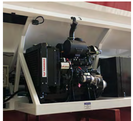
YANMAR 4TNV84T diesel engine installed in CRF's SUPA bin
