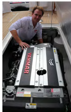
Yanmar 8LV installed in Tasman Boats
