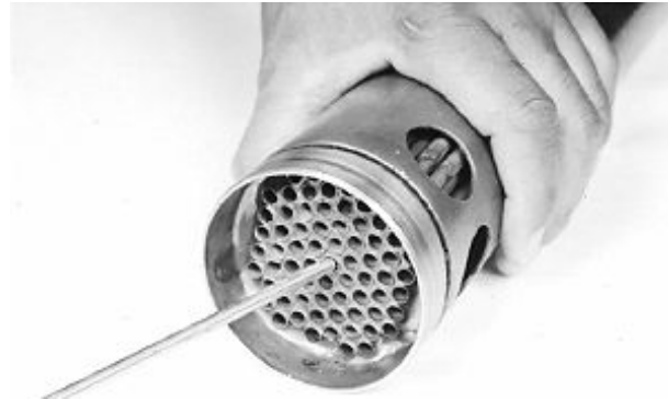
Clean Heat Exchanger
